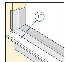
I. **When required for adequate sill support,** attach the optional aluminum sill support or wood blocking to the exterior of the box plate to support the edge of the door sill (1I). Place the sill support flush with the subfloor.
