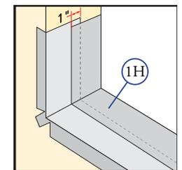
H. **Apply sill flashing tape #2.** Cut a piece of flashing tape 12" longer than the opening width. Apply at the bottom, overlapping tape #1 by at least 1". DO NOT allow the tape to extend past the interior face of the framing (1H). If the wall depth is greater than 5", add a third piece of flashing tape. The flashing tape should come to within 1" of the interior face of the framing.
