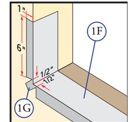
G. **Tab the sill flashing tape and fold.** Cut 1" wide tabs at each corner (1/2" from each side of corner) (1G). Fold tape to the exterior and press firmly to adhere it to the water resistive barrier.
