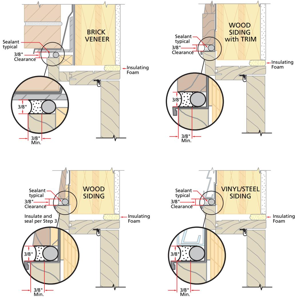
A. **Insert backer rod into the space around the door** as deep as it will go. This should provide at least a 3/8" clearance between the backer rod and the brickmould (5A).
