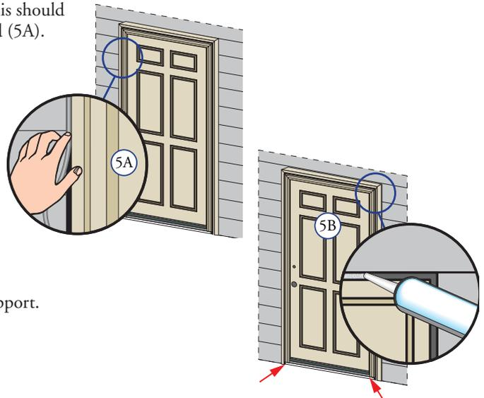
C. **Apply a bead of sealant** between the exterior edge of the sill and the sill support.
