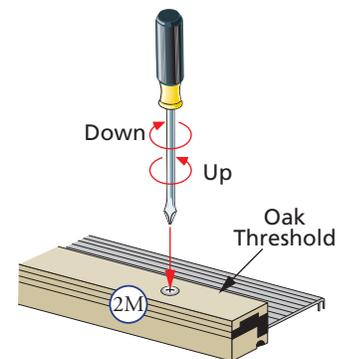
M. **If needed, the height of the threshold can be adjusted** to achieve appropriate contact with the door sweep. Using a #3 Phillips screwdriver, turn the adjustment screws clockwise to lower the threshold, and counter-clockwise to raise the threshold (2L).
