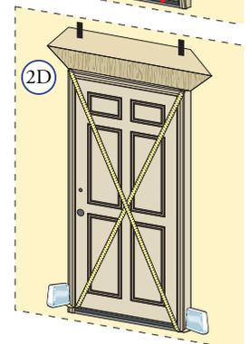
E. Carefully open the door panels and remove all shipping spacers.
