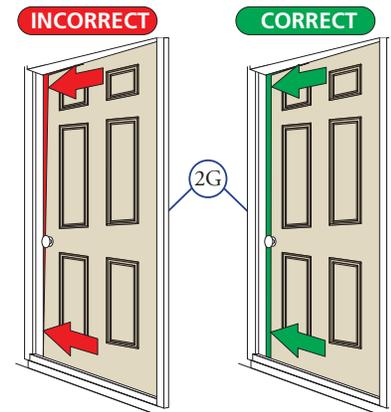
H. **Drive a 10d galvanized finish nail or 3" screw through the frame lock jamb, approximately 6" from the top and bottom,** through the shims and into the structural framing.
