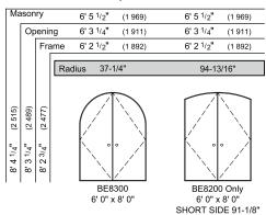
For Out-Swing units with standard bumper sill, subtract 1-3/8" from each of the height measurements. For In-Swing/Out-Swing units with ADA sill, subtract 7/8" from each of the height measurements.
