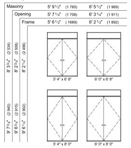
For Out-Swing units with standard bumper sill, subtract 1-3/8" from each of the height measurements.
