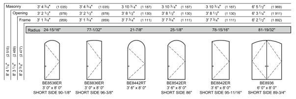
For Out-Swing units with standard bumper sill, subtract 1-3/8" from each of the height measurements. For In-Swing/Out-Swing units with ADA sill, subtract 7/8" from each of the height measurements.
