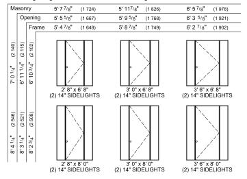
For Out-Swing units with standard bumper sill, subtract 1-3/8" from each of the height measurements.
