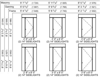
For Out-Swing units with standard bumper sill, subtract 1-3/8" from each of the height measurements.
